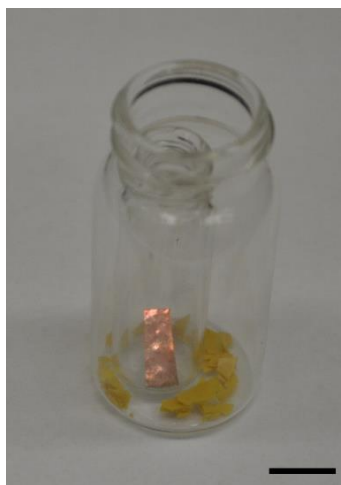
Figure 2.1. Photo of the reaction setup before sealing and injection of dilute H 2 SO 4 solution. The double vials ensure that the graphene sample is only exposed to H 2 S gas which is generated in situ , not any liquids or solids. Scale bar: 1 cm.
